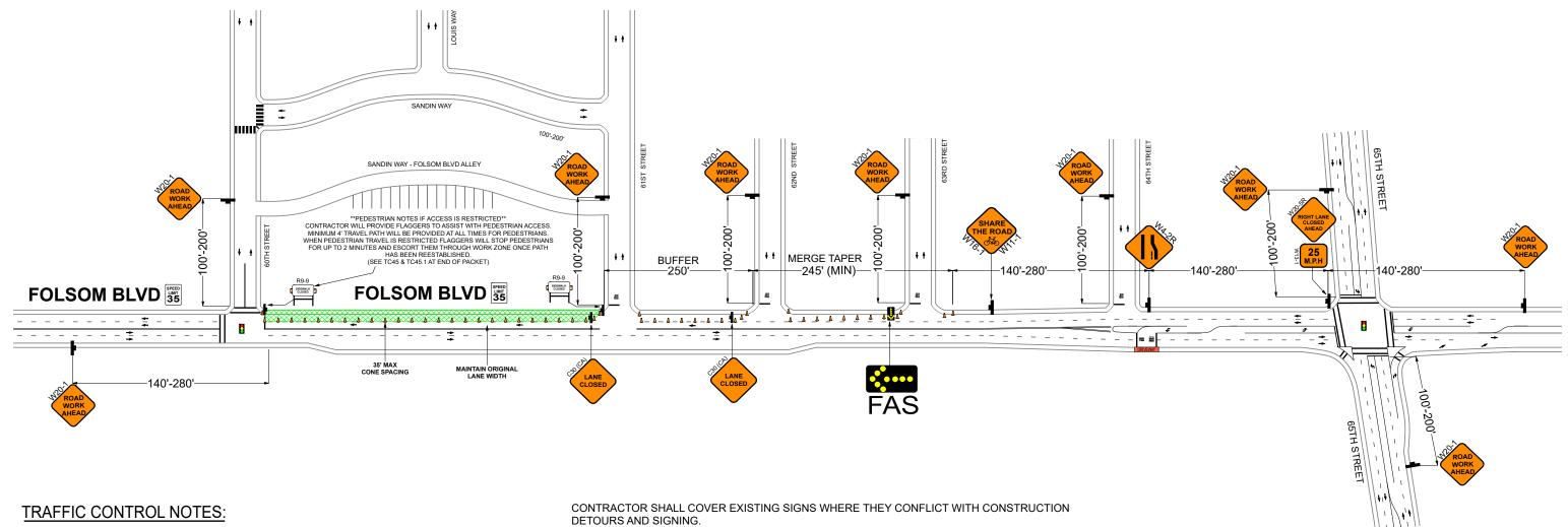
IT IS THE RESPONSIBILITY OF THE CONTRACTOR PERFORMING WORK TO INSTALL AND MAINTAIN THE TRAFFIC CONTROL DEVICES AS SHOWN HEREIN, AS WELL AS ANY SUCH ADDITIONAL TRAFFIC CONTROL DEVICES AS MAY BE REQUIRED TO INSURE THE SAFE MOVEMENT OF VEHICULAR AND PEDESTRIAN TRAFFIC THROUGH OR AROUND THE WORK AREA AND PROVIDE MAXIMUM PROTECTION AND SAFETY TO CONSTRUCTION WORKERS.
