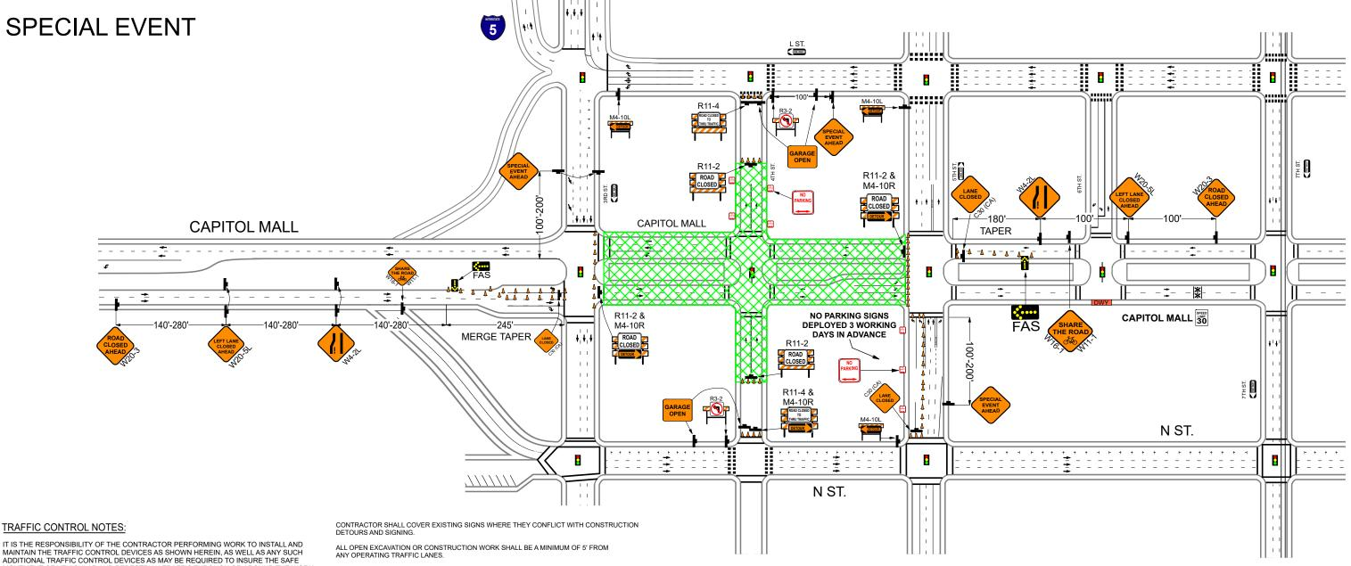
MAINTAIN THE TRAFFIC CONTROL DEVICES AS SHOWN HEREIN, AS WELL AS ANY SUCH ADDITIONAL TRAFFIC CONTROL DEVICES AS MAY BE REQUIRED TO INSURE THE SAFE MOVEMENT OF VEHICULAR AND PEDESTRIAN TRAFFIC THROUGH OR AROUND THE WORK AREA AND PROVIDE MAXIMUM PROTECTION AND SAFETY TO CONSTRUCTION WORKERS.
