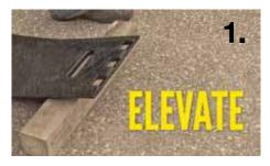
Put the 4x4 under the slotted end of the first section.
