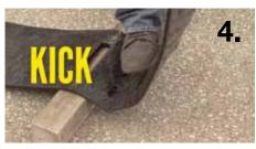
**KICK** the section in your hand to fully engage the channel on the rod.
